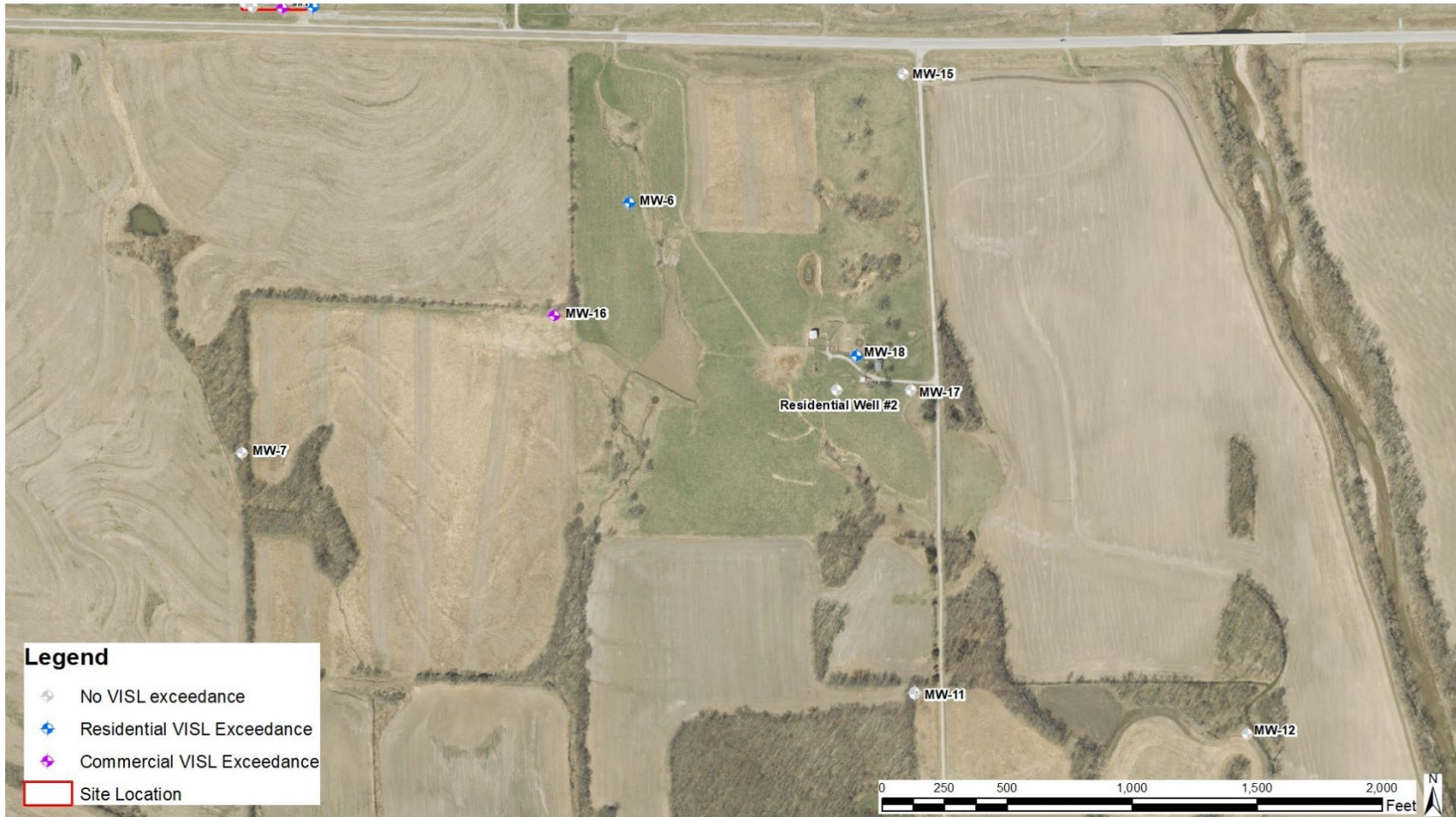
Figure 10. Vapor intrusion risk assessment results based on groundwater carbon tetrachloride (CTC) / chloroform (CF) concentrations, southeast of site.
